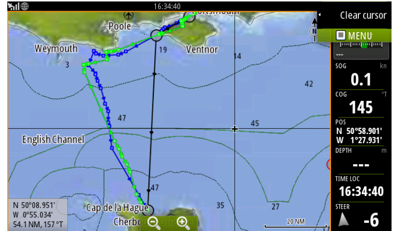
PredictWind optimised routes, based on weather conditions and currents, live on a Zeus MFD
